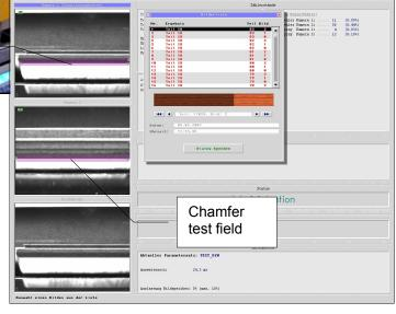
BEVELchecker for chamfer testing on laminate planks. Testing of both painted and foil-coated planks is possible.
